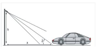
In both the vertical and the horizontal placement, the angle between the camera lens and the farther lane border must be less than 30°. Ensure the snapshot distance (x) of the camera is greater than 1.7 times the height (h) of the camera (x > 1.7 x h) for optimal license plate images.
