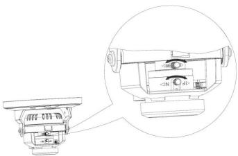
2) Lock the levers, and then put the dome<sup>⑤</sup> back on and fasten the locking screws
