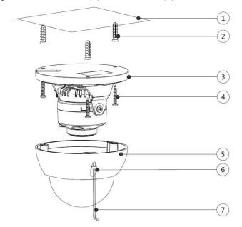
Figure 3-3-3 Model B (1) and Model B (2) installation
