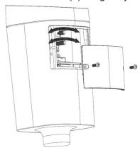
5) Lock the levers and bottom cover, and then fasten the locking screws.
