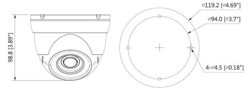
Figure 2-2 Model B (1) and Model B (2) (mm [in.])
