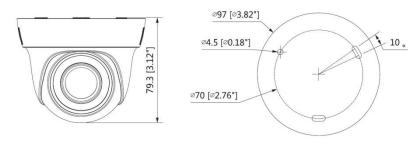
Figure 2-7 Model G (1) and Model G (2) (mm [in.])
