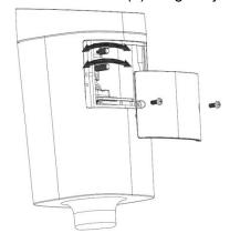
3) Lock the levers and bottom cover, and then fasten the locking screws.
