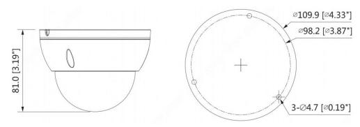
Figure 2-3-2 Model B (1) and Model B (2) (mm [in.])
