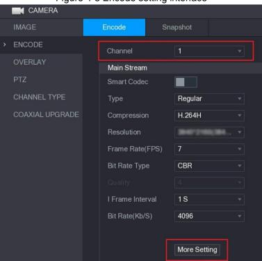
Figure 4-3 Encode setting interface
