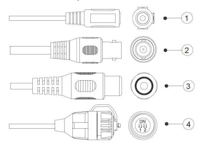
For more information about cable ports, see Table 2-1; for the operation method of ④ (DIP switch), see Table 2-2.
