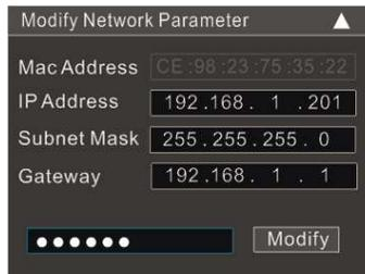
For example, the IP address of your computer is 192.168.1.4. So the IP address of the camera shall be changed to 192.168.1.X. After modification, please enter the password of “admin” which is set in the device activation interface in advance and then click the “Modify” button to change the network parameters.
