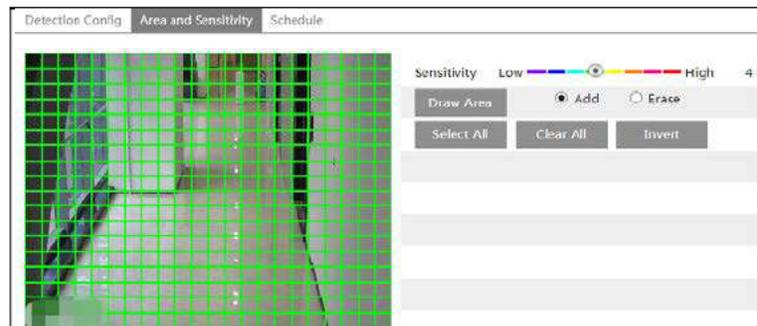
Move the “Sensitivity” scroll bar to set the sensitivity. Higher sensitivity value means that motion will be triggered more easily.
