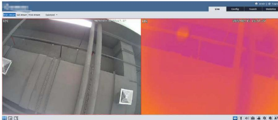
Plug-in free live view: when the main stream is set over 1080P, only the sub stream or third stream tab can be displayed on the above interface by default.
