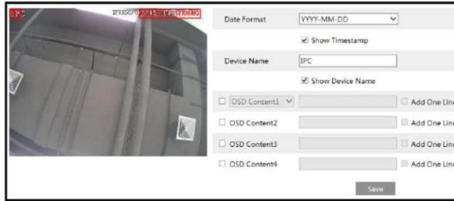
Set time stamp, device name, OSD content and picture overlap here. After enabling the corresponding display and entering the content, drag them to change their position. Then click the “Save” button to save the settings.
