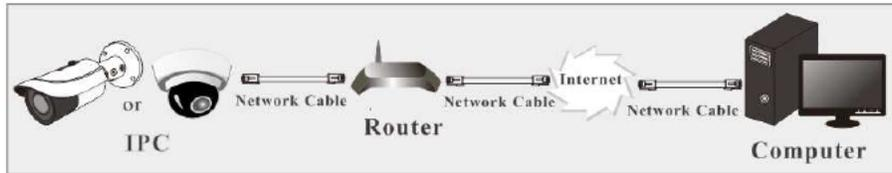
① Make sure the camera is connected to the local network and then log in the camera via LAN and go to Config→Network→Port menu to set the port number.
