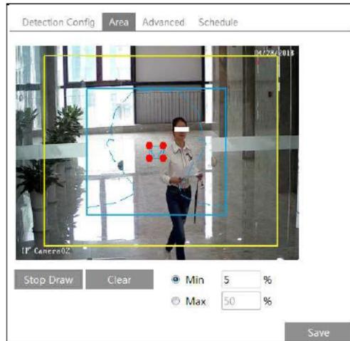
Click “Draw Area” and drag the border lines of the rectangle to modify its size. Move the rectangle to change its position. Click “Stop Draw” to stop drawing the area. Click “Clear” to clear the area. Then set the detectable face size by defining the maximum value and the minimum value (The default size range of a single face image occupies from 3% to 50% of the entire image).
