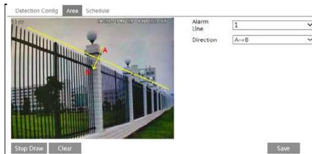
Set the alarm line number and direction. Up to 4 lines can be added. Multiple lines cannot be added simultaneously.
