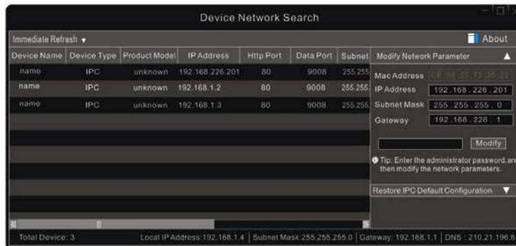
The default IP address of this camera is 192.168.226.201. Click the information of the camera listed in the above table to show the network information on the right hand. Modify the IP address and gateway of the camera and make sure its network address is in the same local network segment as the computer's. Please modify the IP address of your device according to the practical situation.
