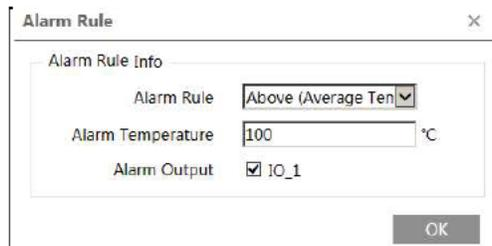
Set the alarm rule, alarm temperature and alarm output. For example, select Alarm Rule as Above (Average Temperature), set the alarm temperature to 100°C and check alarm output. Then alarms will be triggered when the average temperature of the target is higher than 100°C
