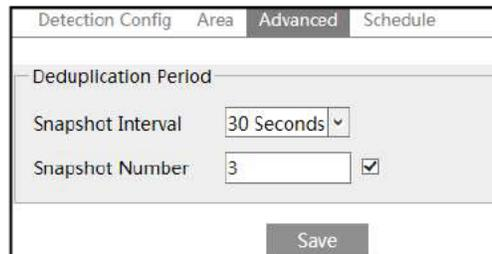
Snapshot Interval: If 5 seconds is selected, the camera will capture the same target once every 5 seconds during its continuous tracking period.
