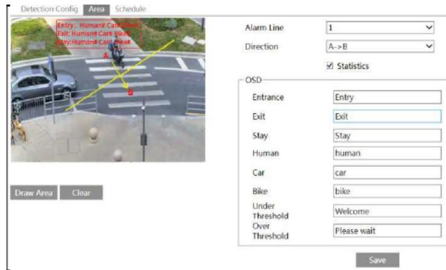
Set the alarm line number and direction. Only one alarm line can be added.
