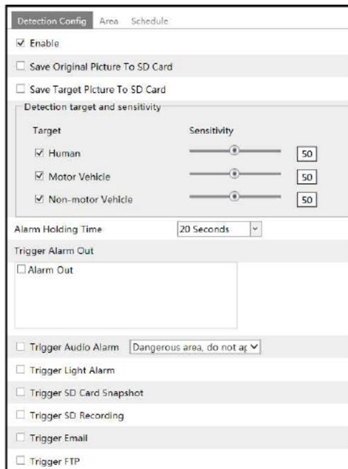
1. Enable intrusion detection and select the snapshot type and the detection target.
