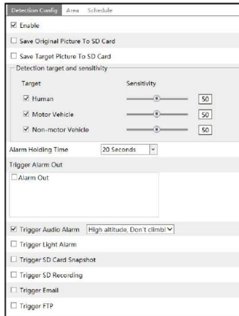
1. Enable line crossing detection and select the snapshot type and the detection target.
