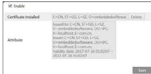
There is a certificate installed by default as shown above. Enable this function and save it. Then the camera can be accessed by entering https://IP: https port via the web browser (eg. https://192.168.226.201:443).
