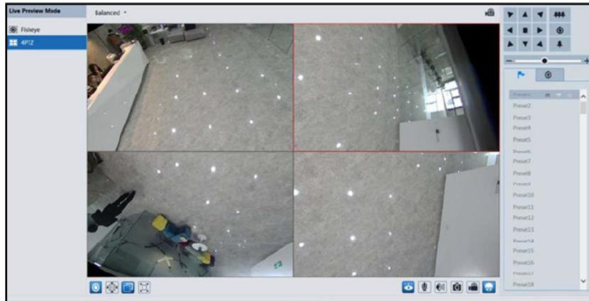
4PTZ fusion view mode: you can view an entire picture formed by 4 small windows. Each small window cannot be controlled by PTZ panel.
