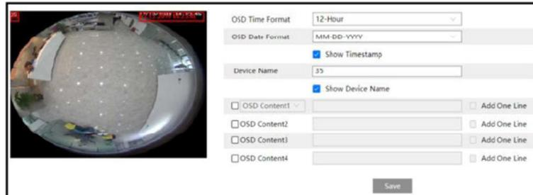
Set time stamp, device name, OSD content and picture overlap here. After enabling the corresponding display and entering the content, drag them to change their position. Then click the “Save” button to save the settings.
