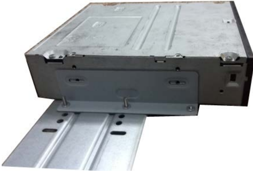
Figure 3-43 Install SATA burner
