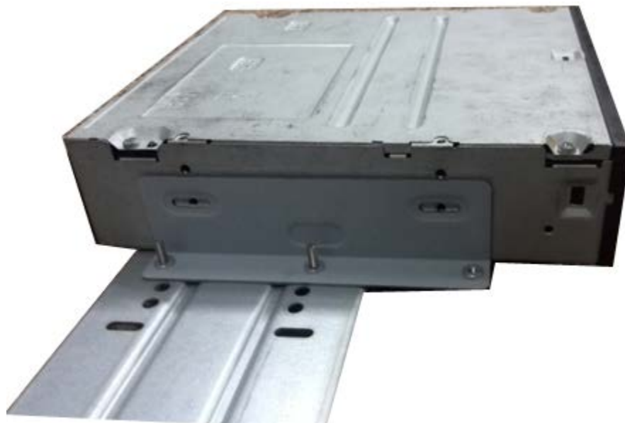
Figure 3-38 Install SATA burner
