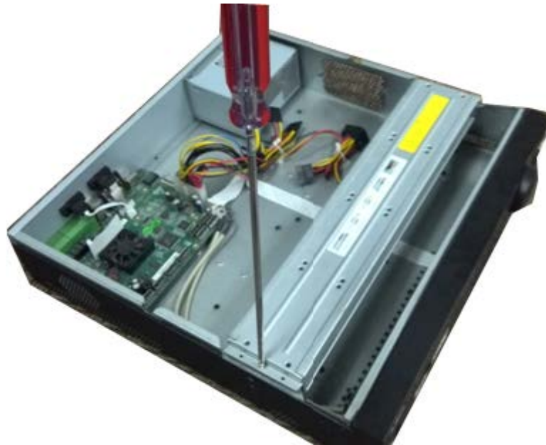
Figure 3-36 Open the top cover
