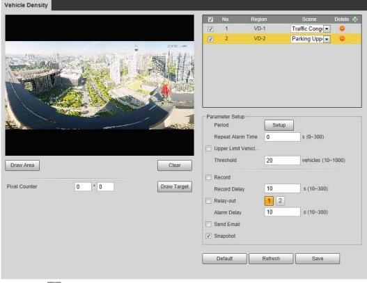
Figure 5-70 Vehicle density (parking upper limit)
