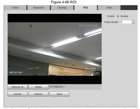
Step 2 Select the Enable check box, draw the area on the image, and then configure the image quality of ROI.
