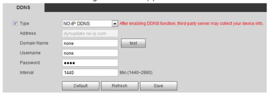
Step 2 Select **Type**, and configure the parameters as needed.
