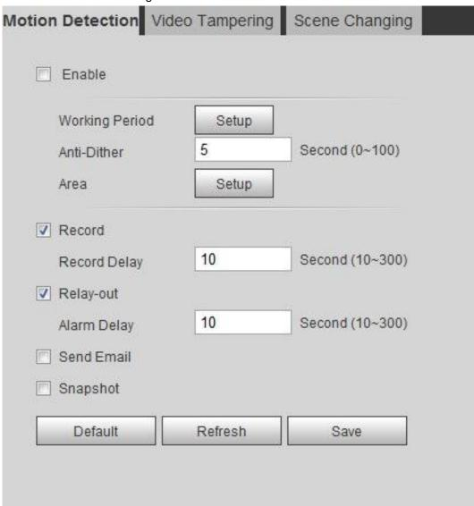
Figure 5-21 Motion detection
