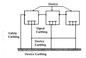
Mixed ground: The mix ground consists of the feature of the one-point ground and multiple-point ground. For example, the power in the system needs to use the one-point ground mode while the radio frequency signal requires the multiple-point ground. So, you can use the following figure to earth. For the direct current (DC), the capacitance is open circuit and the circuit is one-point ground. For the radio frequency signal, the capacitance is conducive and the circuit adopts multiple-point ground.
