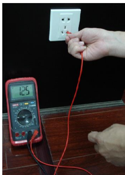
Appendix Figure 7-6 Check live cable connection
