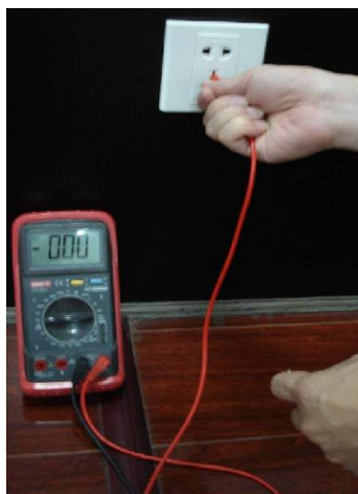
Appendix Figure 7-5 Check earth cable connection
