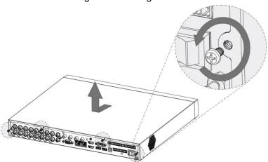
Step 2 Put two screws on the HDD and twist one turn.
